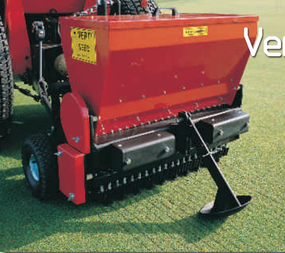
The Verti-Seed is designed for the professional user who wants precision control of dosage and depth, ensuring maximum germination for all seed types. The Verti-Seed's unique action provides direct seed contact with the soil which ensures good germination rates, all this at speeds of up to 16 km/h.
